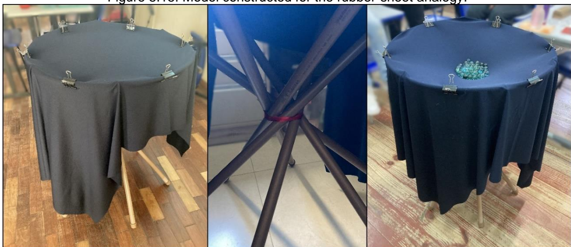
Figure 5.15: Model constructed for the rubber-sheet analogy.
